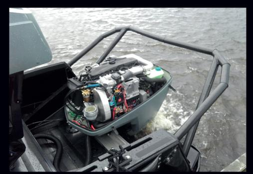
The OXE300 is the most powerful unit in the OXE product line, meeting the demand of users who require high speed and torque capacity for their operations. The twin turbos and the specifically designed gearbox has been developed to withstand the increased torque and power of the 3.0 L aluminum powerhead, providing peak torque at 1750 rpm. Primary customers for the OXE300 are Governmental, Transportation, Search and Rescue and other marine applications with high-speed and load demands.
